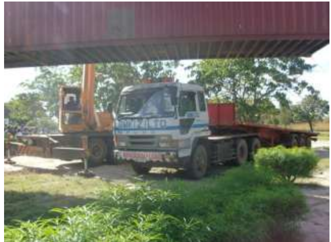
Crane lifting container off truck
